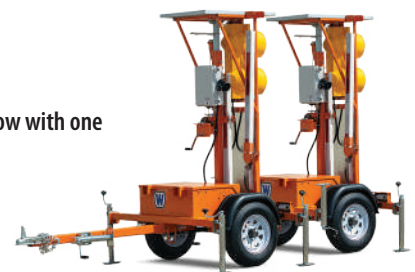
Drawbar tandem tow with two drawbars and hitches
