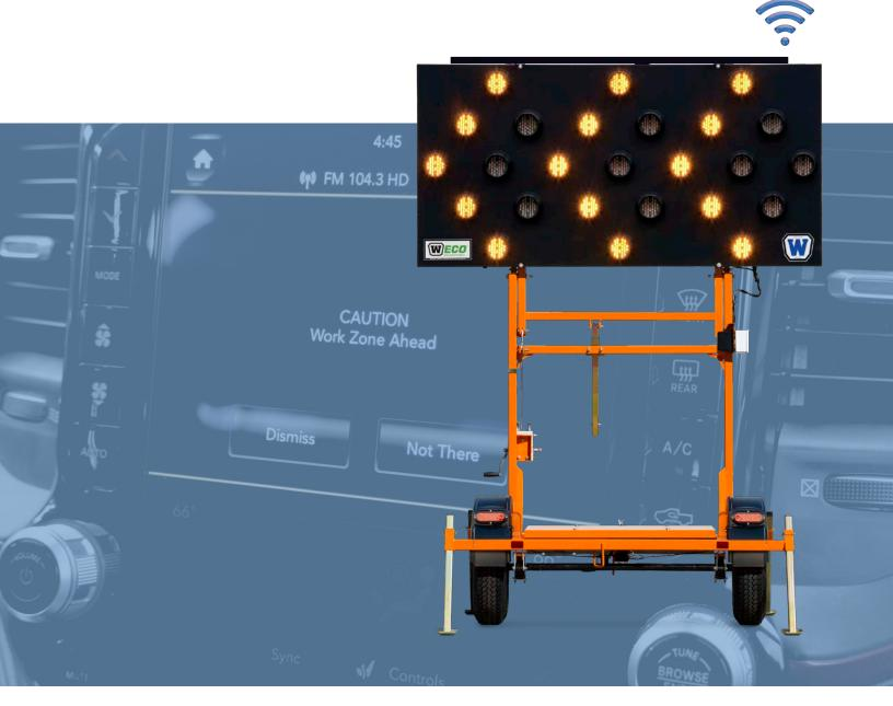
Connected arrow boards send digital alerts to give drivers additional time to move over, slow down and avoid collisions.
